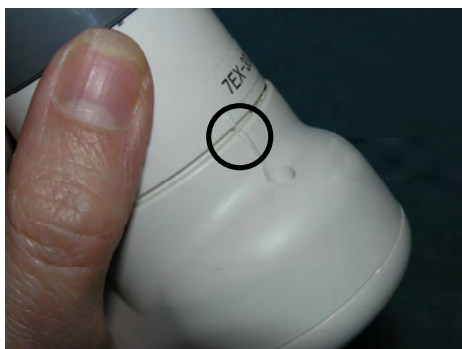
Positions of index marks on lens and camera body before the lens is twisted into place
