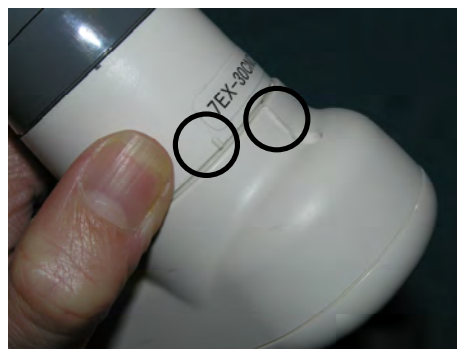
Positions of index marks after lens has been twisted into place and is securely attached
