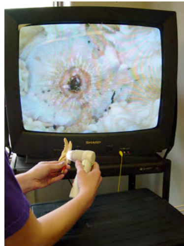
Viewing sea star with contact tip depressed. When the contact tip is depressed, the scope can see further into the sea star, bringing the mouth into focus.
