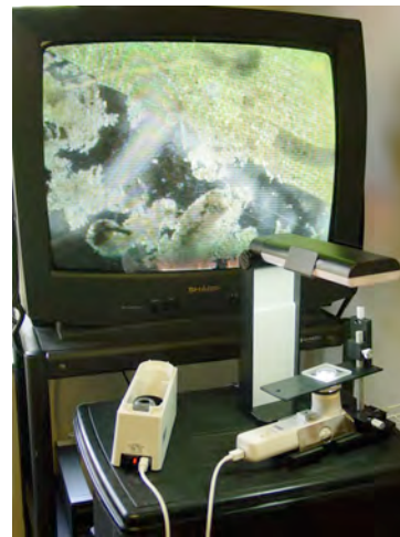
Water sample with lamp and light blocker. Colors in the sample are much more clearly seen.
