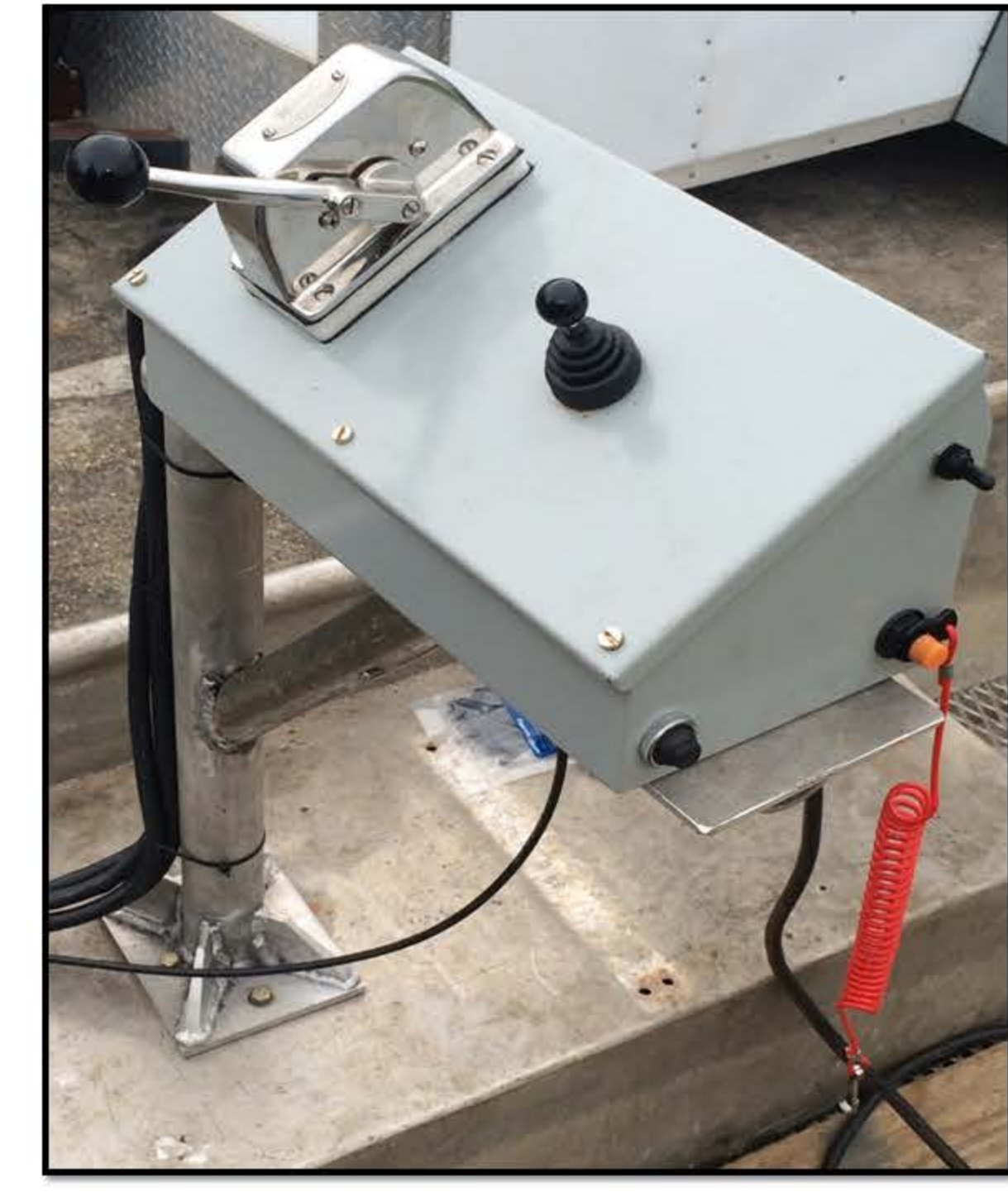
Neutral start-in-gear and kill switch provide safety features for the prototype
