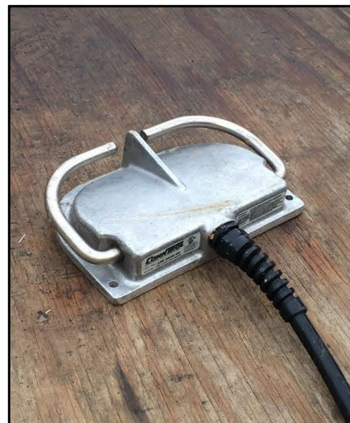
Foot pedal controls motor direction and allows all hands for crawfishing
