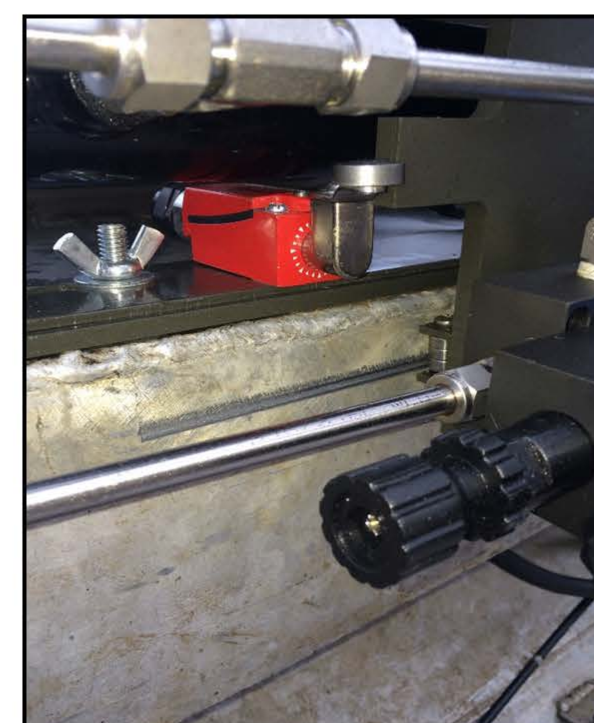
Limit switches allow the motor to return to center
