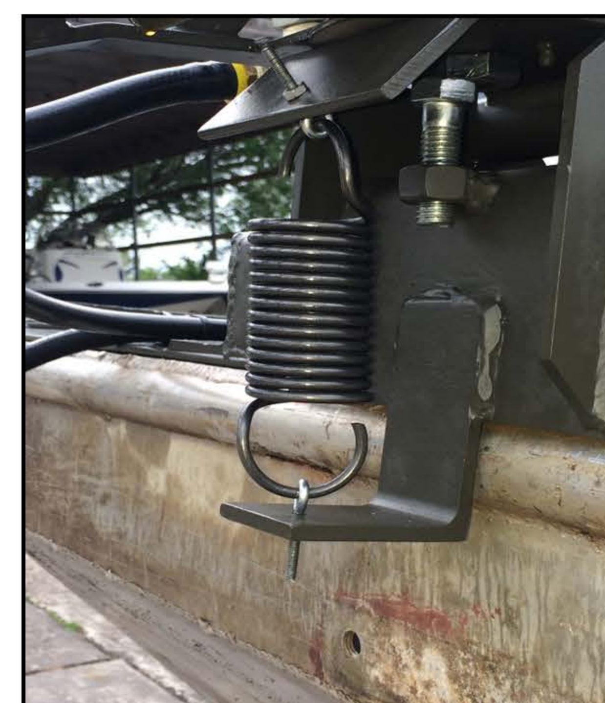
Compression spring to keep the motor in the water at all times
