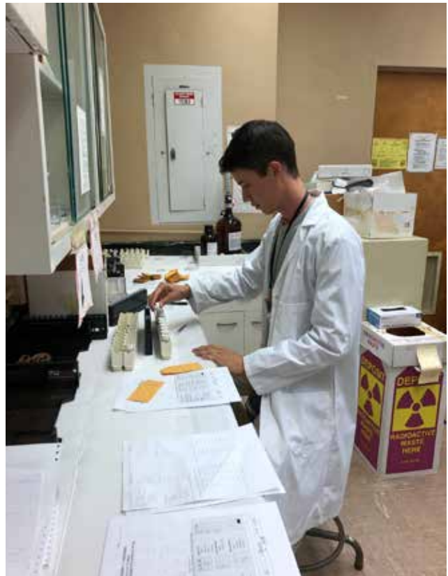
RSO lead technical assistant Adam Curet prepares swipe samples to quantify radioisotopes using a liquid scintillation counter.
